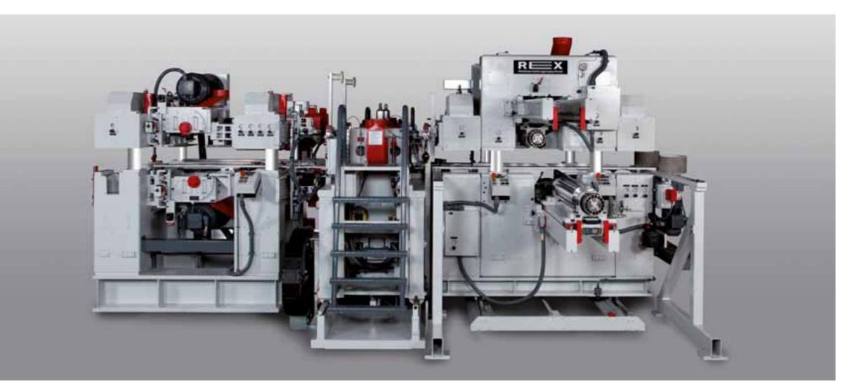
SUPERMASTER 10/41 -WW- for the production of high quality KVH, Duo/Trio Lam, BSH and profiling boards with high speed. Machine shown with profiling and sawing spindles.
